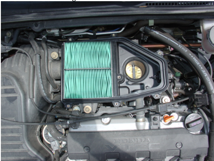
Top View of air filter (air enters from the under side of filter)
