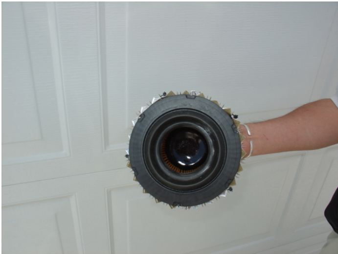
Eco Charge ICB encircles the entire air filter
